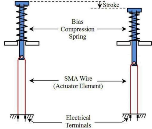
Figure 3. ACTUATOR CONFIGURATION
